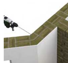
Reconnecting Partition Wall
